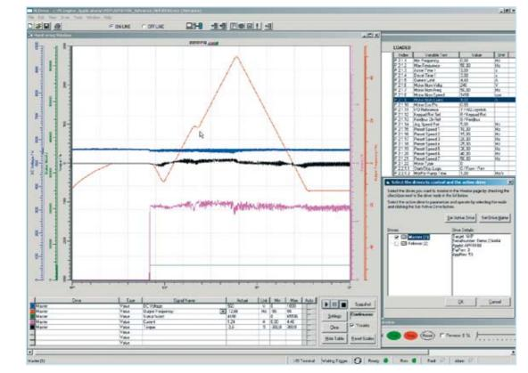
**Graphical trend** screen for simultaneously monitoring of user-specified variables.
